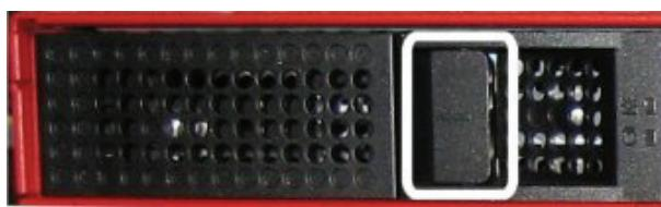
3. Pull the tab outward to release the hinged arm on the hard drive.
