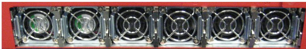
3. Grasp the two vertical handles on the fan you want to replace. Then pull the fan straight out.
