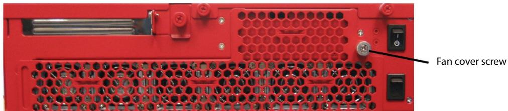
2. Grasp the screw and slide the fan cover to the left to remove it.
