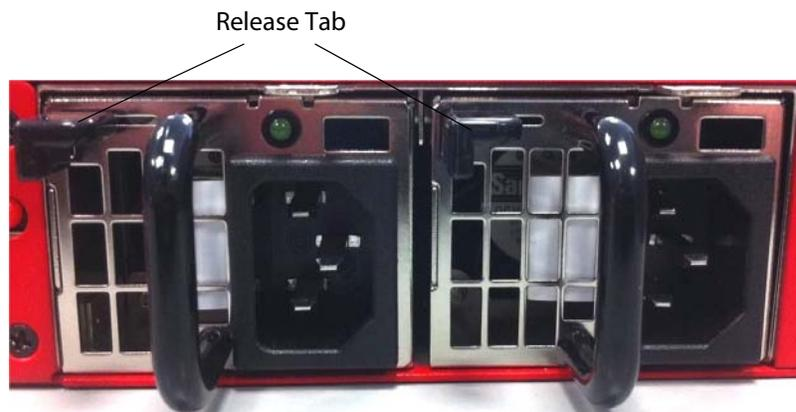
3. Remove the failed power supply.
