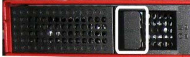
2. Pull the tab outward to release the hinged arm on the hard drive.
