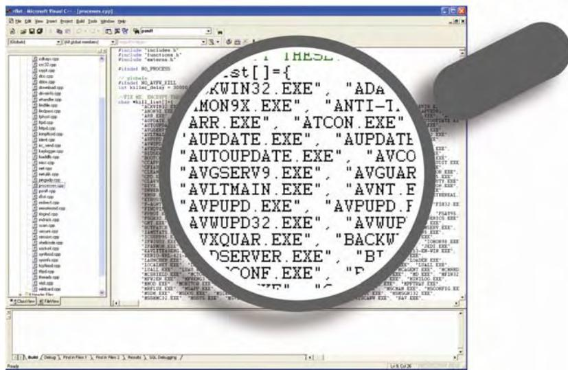
This screen capture comes from Rxbot, commonly found in the wild. In the left panel, each file is another exploit. The magnified file, *processes.cpp*, tells the bot which processes on the victim's machine to seek and kill (thus disabling anti-virus). The botmaster simply adds or removes files to change what this bot can do.
