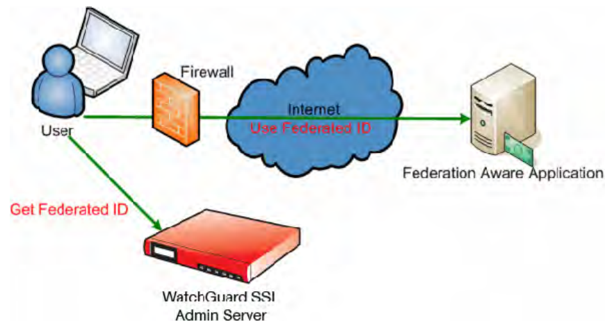
Figure 5: Federated identity allows a single digital identity to be used to access multiple departments, or even businesses, without the need for extra and costly user enrolment. Ideal for sharing identities in B2B partnerships
